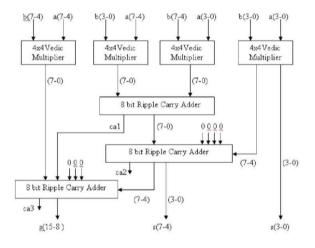
Figure 4[10]: Block Diagram of 8x8 bit Vedic Multiplier.
