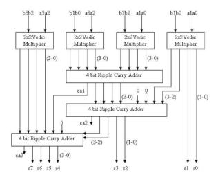
Figure 3[10]: Block Diagram of 4x4 bit Vedic Multiplier.
