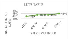
Figure 9 : No.of 4 input LUT comparison of different MAC units.
