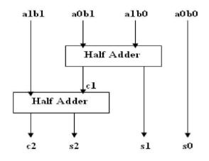
Figure 2[10]:Block Diagram of 2x2 bit Vedic Multiplier.
